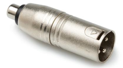
Hosa GXM-133 RCA Female to XLR Male. This adaptor is designed to adapt a phono plug to an XLR input. XLR pin 3 is grounded resulting in an unbalanced signal.
