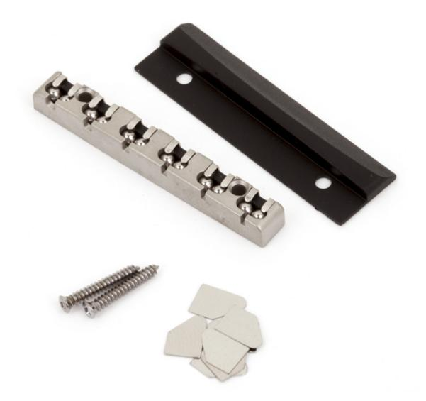
Brushed-chrome LSR roller nut assembly reduces friction that can cause tuning instability. For use on American Deluxe guitars with HSS pickup configuration; also fits older Strat Plus models with included Wilkinson® adapter. For string gauges from .008 to .056. Includes instructions, mounting hardware, shims and Wilkinson® adapter. Note that modification may be required for correct installation. Right-hand only.
