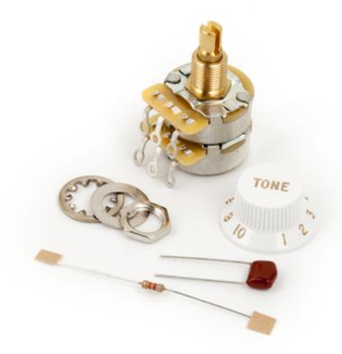
The Treble Bass Expander (TBX) is a stacked and detented 250K/1Meg potentiometer that expands your tonal palette. It functions as a standard tone control from 1 to 5, after which it decreases resistance, sending more bass, treble, presence and output to your amp. Mounting hardware and installation instructions included.
