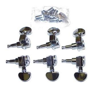
These guitar machines are a triumph in engineering and styling. The housing provides a maximum bearing for worm, gear and string post. Gear ratio is 14:1. Worm and gear are precision-cut for perfect meshing. This eliminates backlash and slippage. Countersunk tension screw permits player to regulate turning tension to any degree. Gear box has a special lubricant for lifetime, trouble-free service. Includes 5/8" washers, bushings and wood screws.
