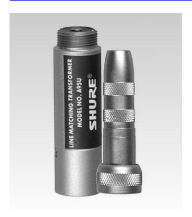
The Shure A95U is a reversible transformer that matches low- or high-impedance microphones to high- or low-impedance inputs. The transformer permits use of very long microphone cables with high-impedance microphones. However, when connecting a high-impedance microphone, limit the cable length between the microphone and the transformer to 4.6 m (15 foot). The cable from the transformer to the low-impedance input can be any desired length.
