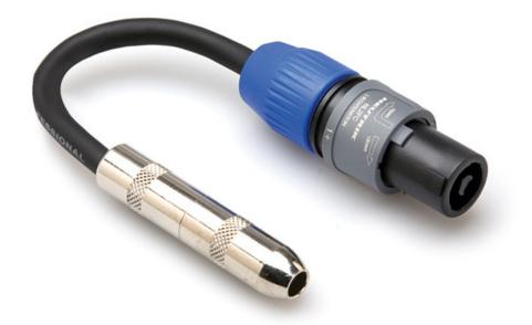
Hosa GSK-116 Speaker Adaptor with Neutrik Speakon Connector on One End and 1/4'' Female on the Other. 16AWG, Approximately 6 inches long.
