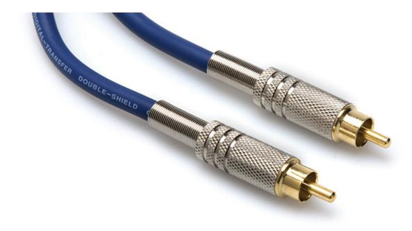
Hosa DRA-503 Double Shielded 75ohm Coax Cable with Gold Plated RCA Connectors. The DRA-500 series cables are designed specifically for S/PDIF. They are also great for use as a composite video cable.
