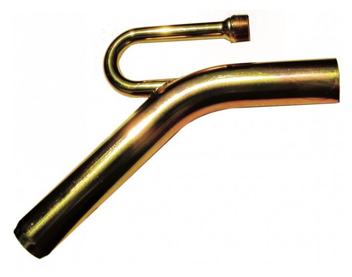
This suction nozzle works with 2.5 inch suction hose and has a net weight of 3.5 pounds. A 1.25 inch pressure hose is easily secured to the nozzle with a 1.25 inch threaded coupling.
