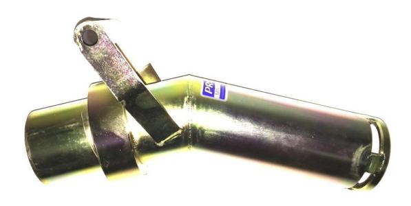
Proline's unique swivel seal is less prone to seizing from sand than other designs. The tip includes a high carbon steel wear ring which is spaced out from the nozzle body to increase dredge capacity and to make it easier to remove large rocks from the tip. This nozzle is built to last!
