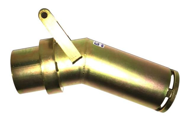
Proline's unique swivel seal is less prone to seizing from sand than other designs. The tip includes a high carbon steel wear ring which is spaced out from the nozzle body to increase dredge capacity and to make it easier to remove large rocks from the tip. This nozzle is built to last!
