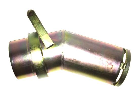
Proline's unique swivel seal is less prone to seizing from sand than other designs. The tip includes a high carbon steel wear ring which is spaced out from the nozzle body to increase dredge capacity and to make it easier to remove large rocks from the tip. This nozzle is built to last!
