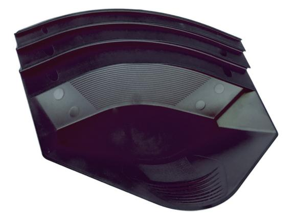
The Gold Claw is very simple to use and the entire process is done under water. Just shake vigorously side to side allowing the gold to settle to the bottom of the pan. Then shake softer while slowly tilting the pan, letting the lighter material fall out of the pan over the large riffles. When down to the heavy concentrates in the pan, transfer the material to the opposite side of the pan and repeat the process till clean gold can be removed from the pan with a snuffer bottle.
