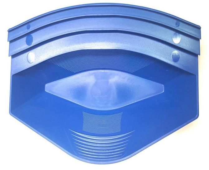
The Gold Claw is very simple to use and the entire process is done under water. Just shake vigorously side to side allowing the gold to settle to the bottom of the pan. Then shake softer while slowly tilting the pan, letting the lighter material fall out of the pan over the large riffles. When down to the heavy concentrates in the pan, transfer the material to the opposite side of the pan and repeat the process till clean gold can be removed from the pan with a snuffer bottle.
