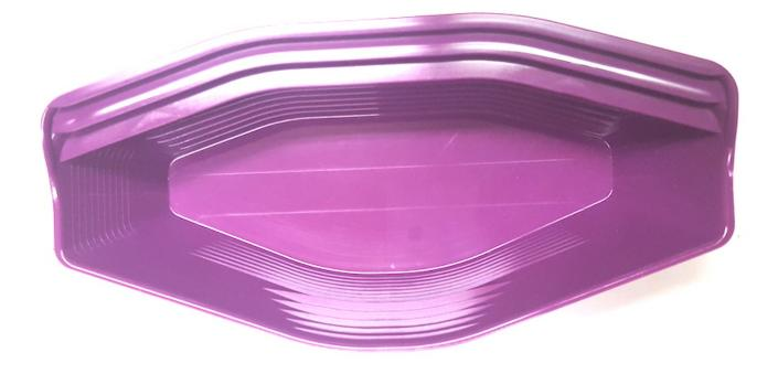
The Gold Claw is very simple to use and the entire process is done under water. Just shake vigorously side to side allowing the gold to settle to the bottom of the pan. Then shake softer while slowly tilting the pan, letting the lighter material fall out of the pan over the large riffles. When down to the heavy concentrates in the pan, transfer the material to the opposite side of the pan and repeat the process till clean gold can be removed from the pan with a snuffer bottle.
