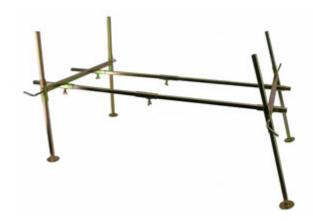
This zinc plated steel sluice stand is 18 inches wide, 36 inches long and designed to hold any sluice up to 10 inches wide (up to 14 inches wide if you do not use the provided clamps). It provides a sturdy platform to use the sluice as a highbanker, power sluice, or dredge. The 1/2 inch square tubular legs are independently adjustable for leveling or setting any angle on any terrain.
