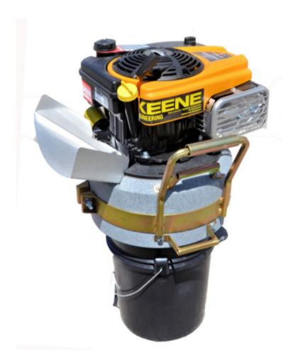
This amazing rock crusher is ideal for the gold prospector interested in a light-weight and economical high-speed machine. Material is gravity fed into the hopper and drops into the center of a high-speed tube. The centrifugal force throws the rock into a hardened steel impact wall at speeds in excess
