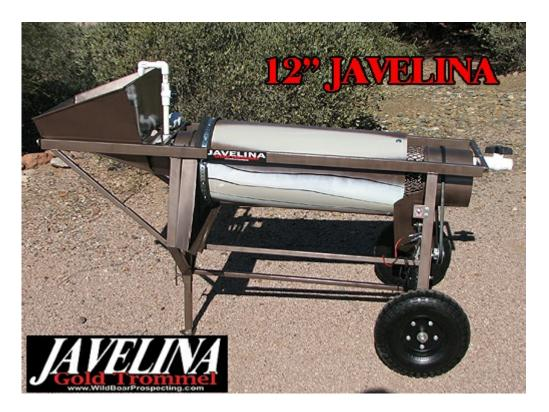
1 ton of material per hour running at optimum performance conditions We run a 1" 37 GPM gas pump on these (not included) 2 Speed 12RPM (low) 19RPM (high) Over 50' of Reverse Helix in the outer barrel 38" Tall x 64" Long x 33" Wide at the base 105 Pounds Hopper is 22" Wide x 17" Long DC Battery Required THIS PRODUCT IS AVAILABLE FOR LOCAL PICKUP ONLY! For Exceptions, Please
