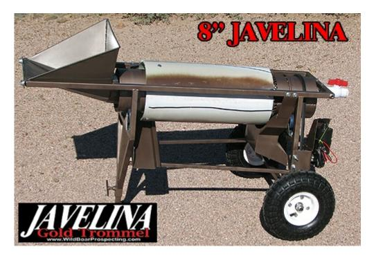
.25 tons of material per hour running at optimum performance conditions Minimum 2500 GPH water pump required (not included)
